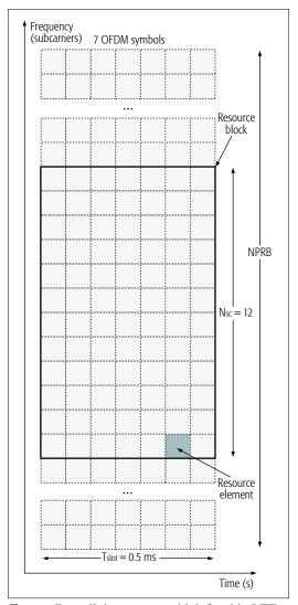
Figure 1. Downlink resource grid defined in LTE.
