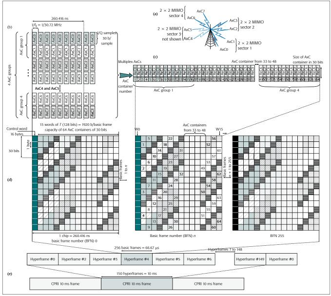
Figure 3. CPRI multiplexing of AxC data in a 2 × 2 MIMO 20 MHz channel use case: a) scenario; b) AxC generation; c) AxC arrangement and serialization; d) basic frame construction; e) hyperframes and 10 ms CPRI frame.
