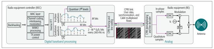
Figure 2. Conceptual explanation of REC/RE functional split.
