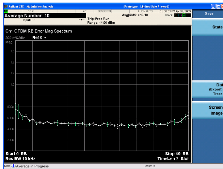
Figure 2 – Residual EVM of LTE test bench for LTE downlink signal with 10 MHz bandwidth and 64QAM subcarrier modulation.
