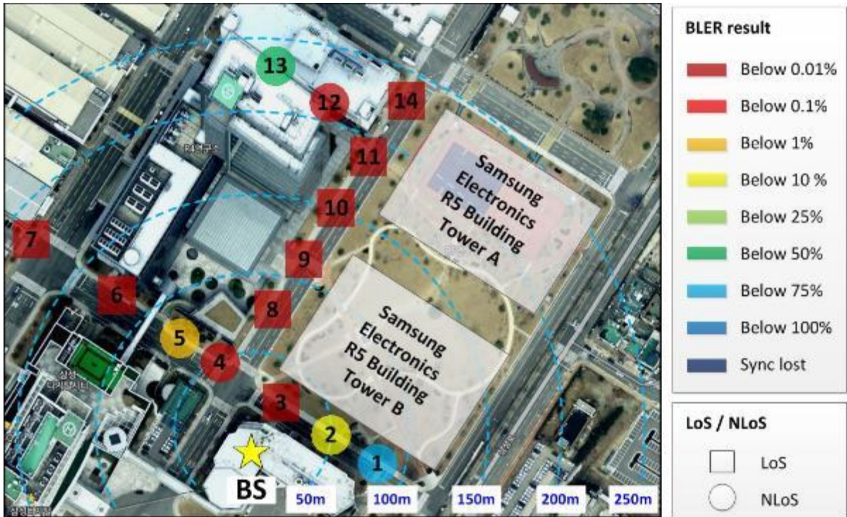
Outdoor coverage test results of bands above 6 GHz beamforming prototype
