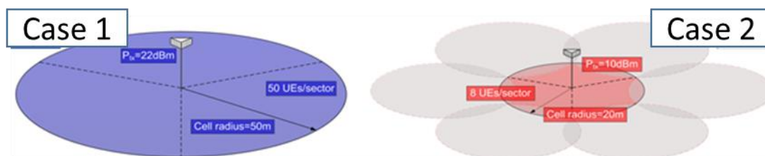
FIGURE A3.4-1 Deployment scenarios for case 1 and case 2
