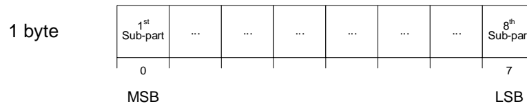
9 10 Figure 31D: 1-byte bitmask format
