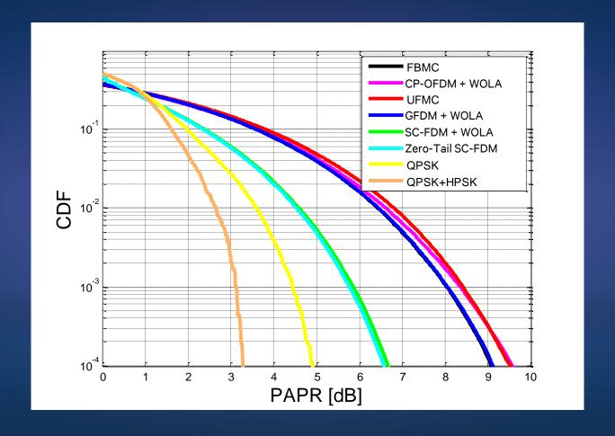
OFDM-based multi-carrier waveform delivers higher spectral efficiency and is suitable for downlink where energy efficiency requirement is more relaxed. Single carrier waveform can be used for other scenarios requiring high energy efficiency.
