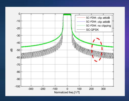
Higher OOB leakage than SC-QPSK due to discontinuities between OFDM transmission blocks
