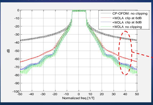
WOLA substantially improves CP-OFDM OOB leakage performance
