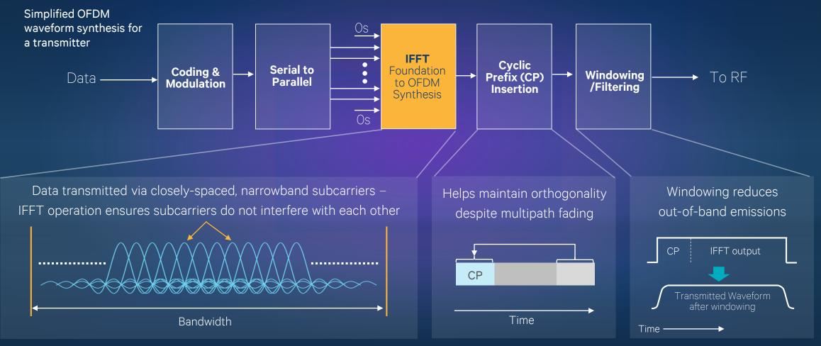
OFDM-based waveforms are the foundations for LTE and Wi-Fi systems today
