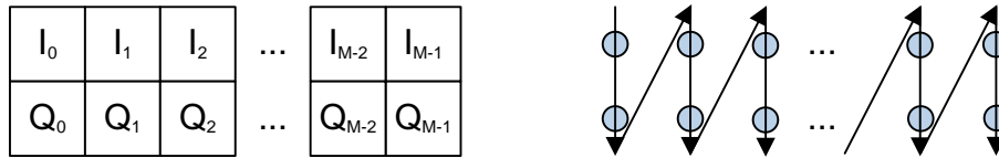
Figure 10: IQ samples within one AxC with oversampling ratio 1
