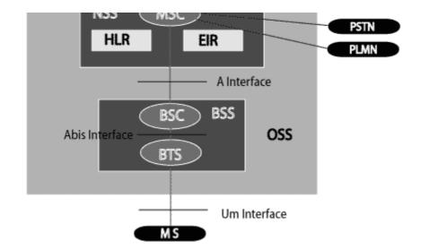
The additional components of the GSM architecture comprise of databases and messaging systems functions:
