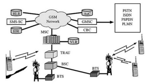
The MS and the BSS communicate across the Um interface. It is also known as the *air interface* or the *radio link*. The BSS communicates with the Network Service Switching *NSS* center across the *A* interface.
