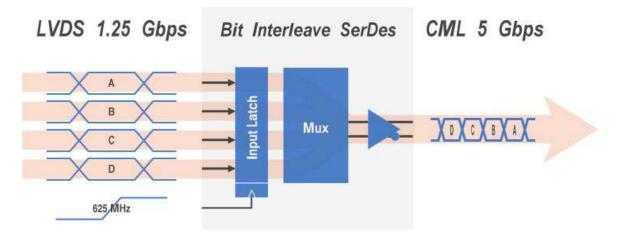
Figure 5. Bit interleaving serializer coding example.
