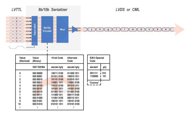
Figure 4. 8b/10b serializer coding example.
