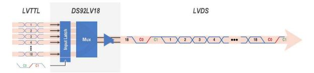
Figure 2. 18-bit embedded clock bits serializer coding example.
