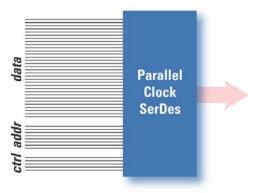
Figure 6. Parallel clock SerDes accommodate traditional wide parallel buses with address and control as well as data signals.
