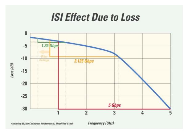
Figure 11. ISI versus signaling rate and run length for a typical FR4 backplane.
