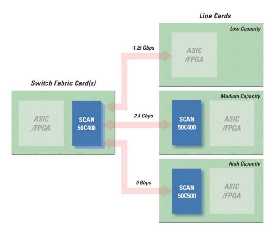
Figure 14. Bit interleaving SerDes router application example.
