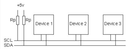
The value of the resistors is not critical. I have seen anything from 1k8 (1800 ohms) to 47k (47000 ohms) used. 1k8, 4k7 and 10k are common values, but anything in this range should work OK. I recommend 1k8 as this gives you the best performance. If the resistors are missing, the SCL and SDA lines will always be low - nearly 0 volts - and the I2C bus will not work.
