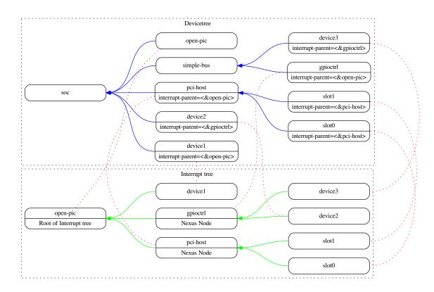
Fig. 2.3: Example of the interrupt tree
