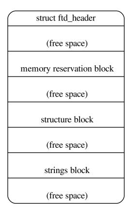
Fig. 5.1: Devicetree .dtb Structure
