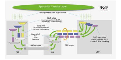
A large part of the functionality providing data connectivity is for supporting flexible deployment of application functions in the network topology as needed for edge computing, which is supported, for example, via three different Session and Service Continuity (SSC) modes or via the functionality of Uplink Classifiers and Branching Points.
