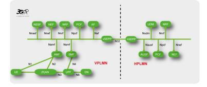
Service based principles apply between the control plane network functions of the Core Network. Further, the 5G system architecture allows network functions to store their contexts in Data Storage Functions (DSF). Functionality for releasing the UE specific Access Network – Core Network transport associations from one AMF and re-binding with another AMF enables separating such data storage also for the AMF. Earlier system architectures had more persistent UE specific transport
